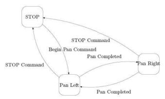
**Figure 3:** The Tekkotsu state machine that drives the robot's constant head panning is quite simple. A command from the laptop-based controller activates the panning which will continue until a STOP command is sent by the laptop.
