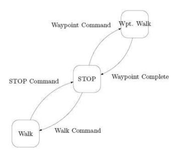
Figure 4: Locomotion is driven by this Tekkotsu state machine. A command from the laptop-based controller either sets the robot on a course specified by a Tekkotsu waypoint or instructs the robot to begin walking in a particular direction until a STOP command is sent.
