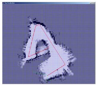
Figure 5: The occupancy grid module builds a map as the robot wanders through the environment. Darker squares indicate a greater likelihood that the area is occupied by an obstacle or a wall.
