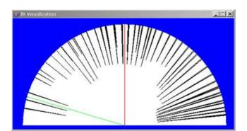
Figure 1: The infrared view module displays data collected from the most recent pan of the robot's head. Lines are drawn from the point at which an obstacle is detected to the bounds of the sensor range to better visualize the robot's perception of its environment.
