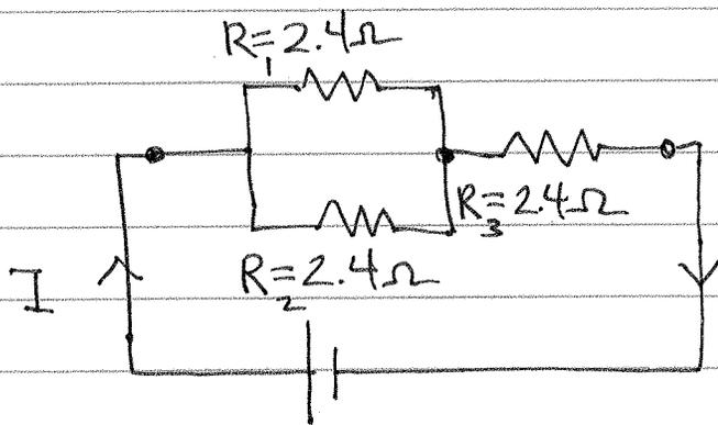
When connected to a source of emf, the entire current  $I$  passes through  $R_3$  while only half as much passes through each of the resistors in parallel ( $R_1$  and  $R_2$  ~~are~~ because they are equal).
