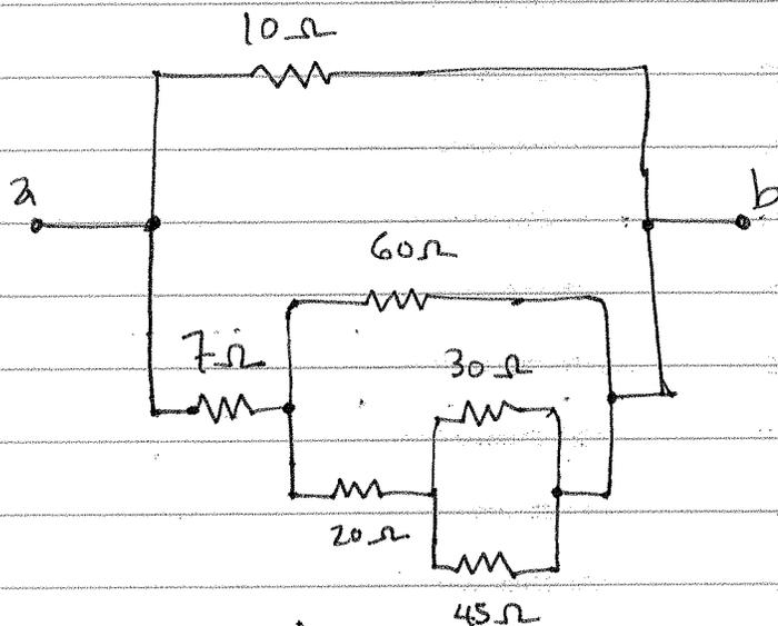
↑ parallel combination is  $\frac{30 \Omega \cdot 45 \Omega}{75 \Omega} = 18 \Omega$
