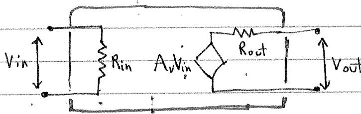
In general input and output resistors should be replaced with impedances that can have imaginary components (capacitance, usually).
