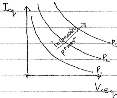
The circuit elements  $V_{cc}$ ,  $R_c$ , and  $R_E$  should be selected so that the load line lies well below the ~~power~~ constant power contour associated with the maximum power dissipation in the transistor.
