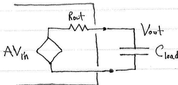
The high frequency half-power point associated with load capacitance is...
