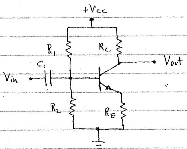
$R_1$  and  $R_2$  form a voltage divider with input  $+V_{CC}$  such that its output,  $V_{BQ}$  ...
