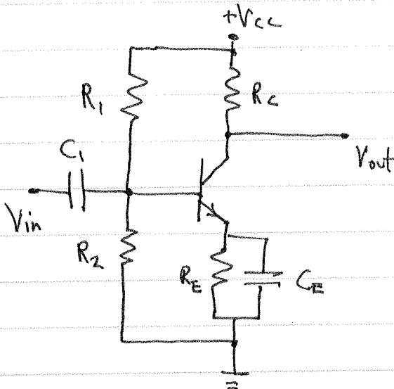
The input impedance of the transistor "looking into" the base is now frequency dependent and the low-frequency roll-off will therefore be affected.
