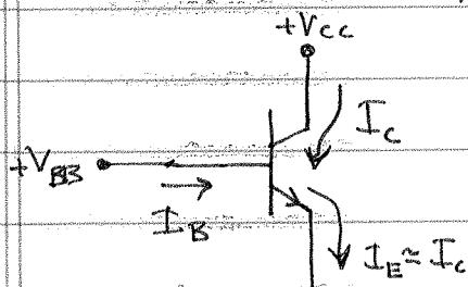
The base-emitter junction is forward-biased,  $V_{BE} > 6V$
