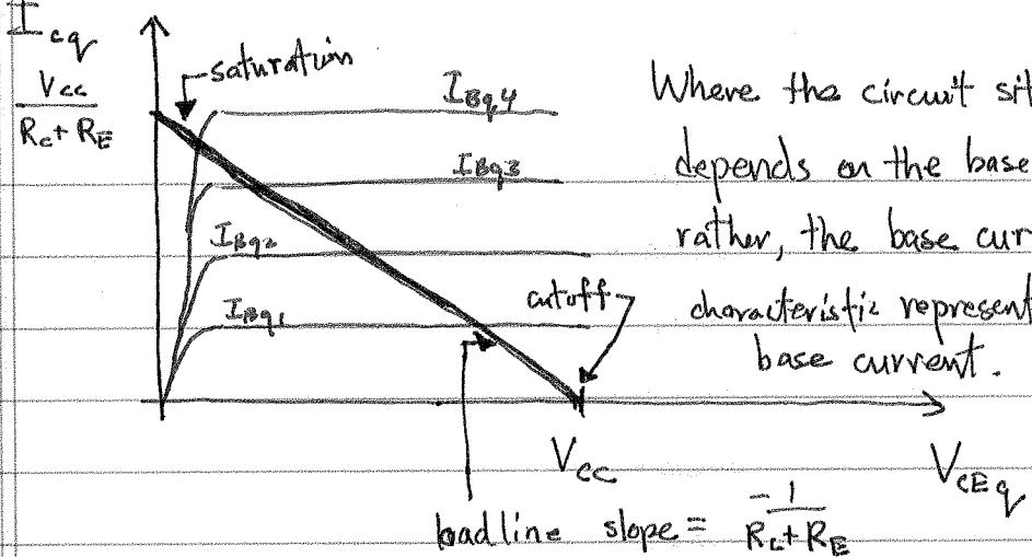
Where the circuit sits on the load line depends on the base-to-emitter bias or rather, the base current. Each horizontal characteristic represents a different quiescent base current.
