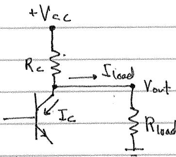
When a load is attached to the output, additional current must flow through  $R_c$  to supply the load.
