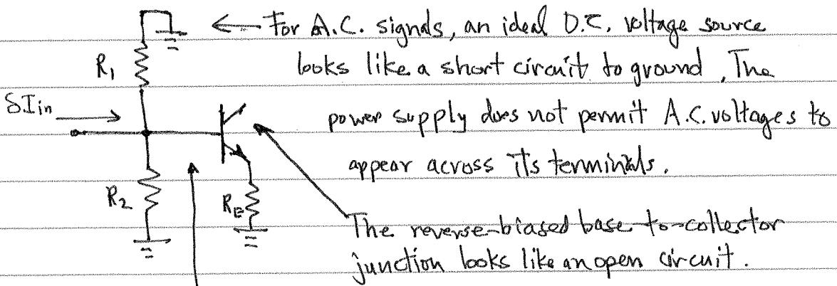
The effective input impedance of the path to the base of the transistor can be obtained from the equation on the bottom of page 3.
