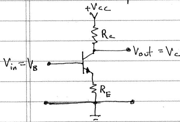
This addition constitutes an application of "negative feedback" and is a sacrifice of gain for other performance characteristics.
