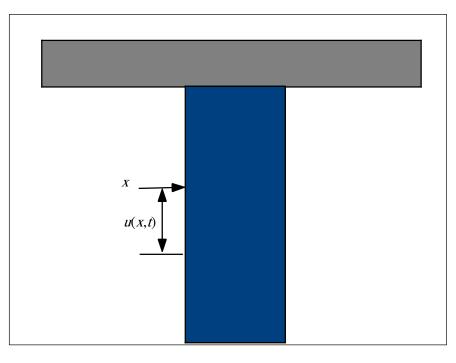
At any given point in time, the portion of the bar labeled x will be found at a location other than x as the bar vibrates. Let u(x,t) stand for the displacement measured from where the portion of the bar at x started at equilibrium. If that portion of the bar is displaced downward from its equilibrium location, u(x,t) will be positive.
