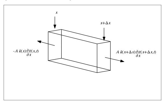
Adding these two net stresses at either end gives the net stress force acting on the entire portion of the bar.
