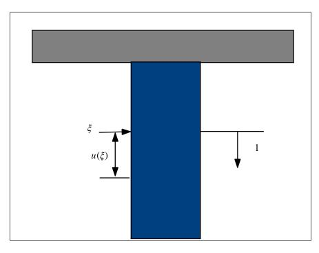
with the modification that the bottom end is now fixed, we see that once again the portion of the bar between x = 0and  $x = \xi$  will experience stretching, while the portion of the bar between  $x = \xi$  and x = l is compressed. This means that bar will "push back" against the external force with two force terms: one is the stress on the upper part of the bar which is being stretched and the other is the stress on the lower part of the bar which is being compressed.
