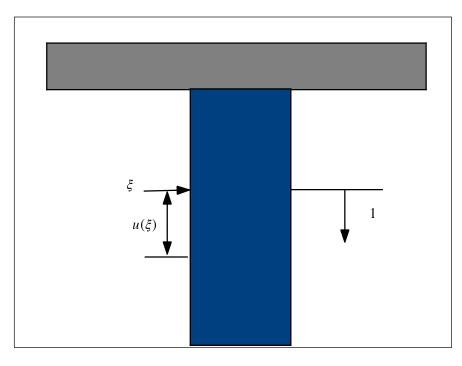
The physical interpretation of this situation is very simple. We are applying one unit of force concentrated over an infinitely thin range of contact centered at  $x = \xi$ . Since the bar has a uniform Hooke's constant of k, we can easily compute how the bar will respond to this situation. The portion of the bar between 0 and  $\xi$  will stretch uniformly in accordance with the underlying physical principle
