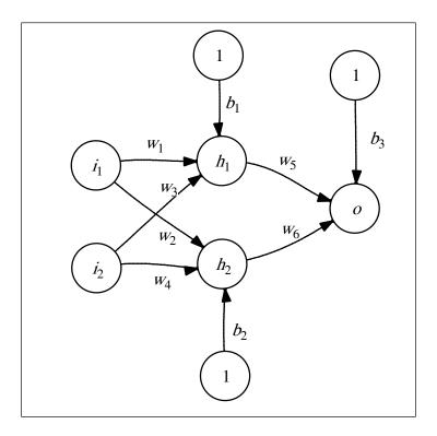
The three units labled with 1s are bias units. These units always output a value of 1. The combination of the bias unit and the weight of the connection connecting it to a unit in the network is to set the threshold for the unit.
