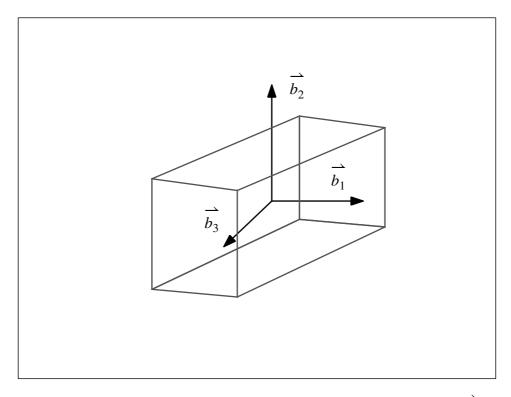
The initial stretching transformation is accomplished by scaling coordinates in the  $\vec{b_3}$  direction up by a factor of two:
